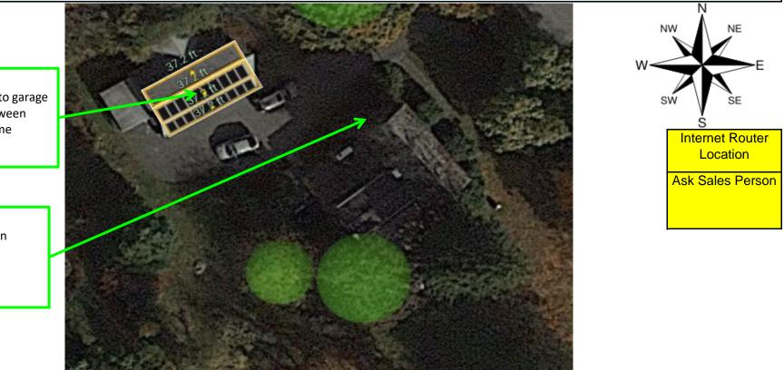
Array 60 amp circuit to garage 2" Conduit between garage and home
