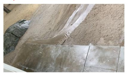
Sandbags added to simulate berm. Positive effect.
