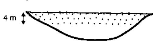
Figure 10.1 Schematic illustration of scum-forming potential changing the cyanotoxin risk from moderate to very high (After Falconer et al. , 1999)
